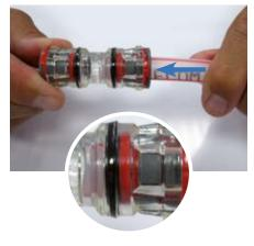
**3. Release of the microduct** is done after removal of the mounted safety clip (if present), by pressing the holding device in the direction of the arrow, as shown in the picture. The microduct can then be pulled out.
